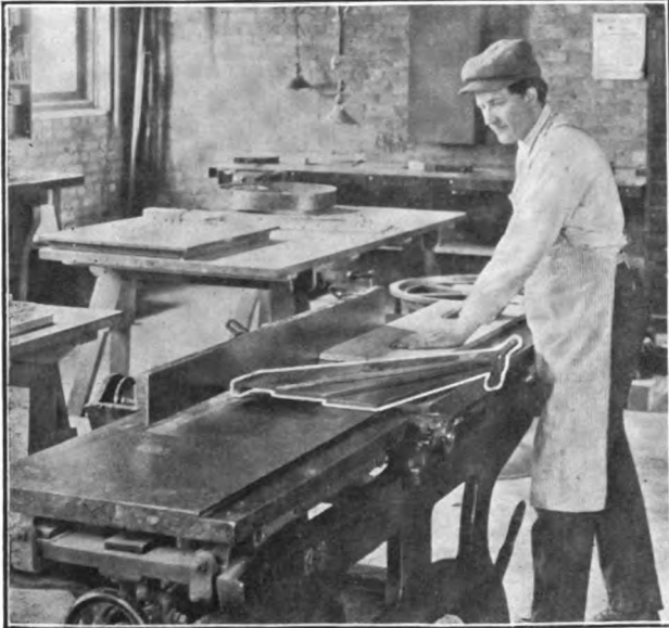
Fig. 12. Shows an automatic wing guard that is composed of three leaves and equipped with a spring so that it automatically returns to its position to entirely cover the knives after the board has passed through.
